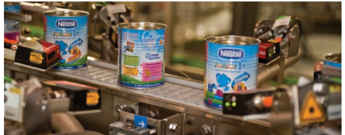
A total of six scanners are used for reading the barcodes
