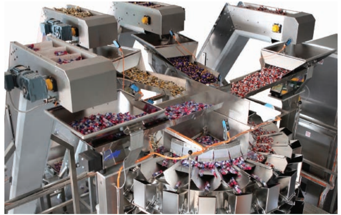
Each weigher is equipped with four separate feed systems
