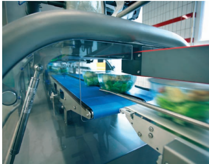
Ishida Europe has designed and installed a complete packing line enabling three to four operators to produce prepared salads
