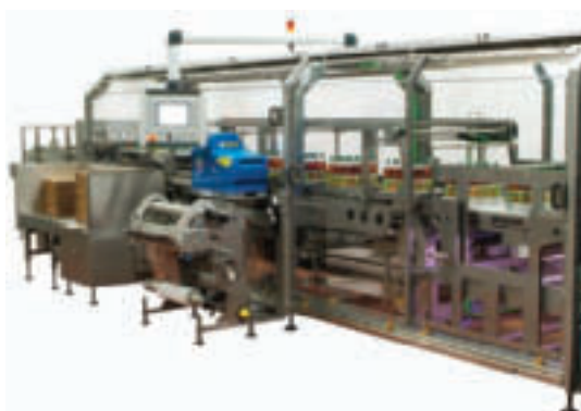
The compact, integrated tray packing and film wrapping machine.
