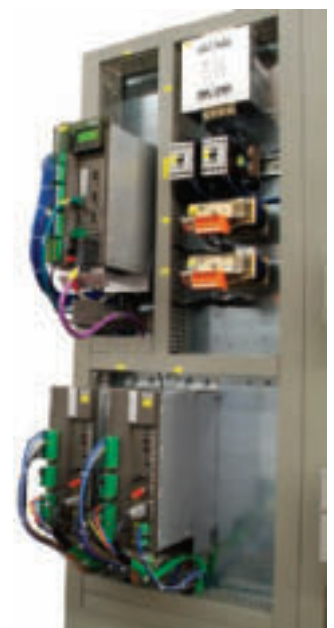
A single ELAU controller (top) and two power suppliers are all that's needed to control 14 servo modules.
