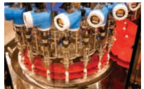
Mengibar flowmeter filler for foaming products
