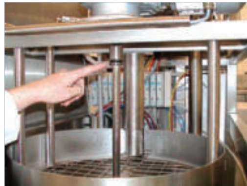
Festo CDVI control valve terminals used in Apple Engineering's automated dough ball filling machine
