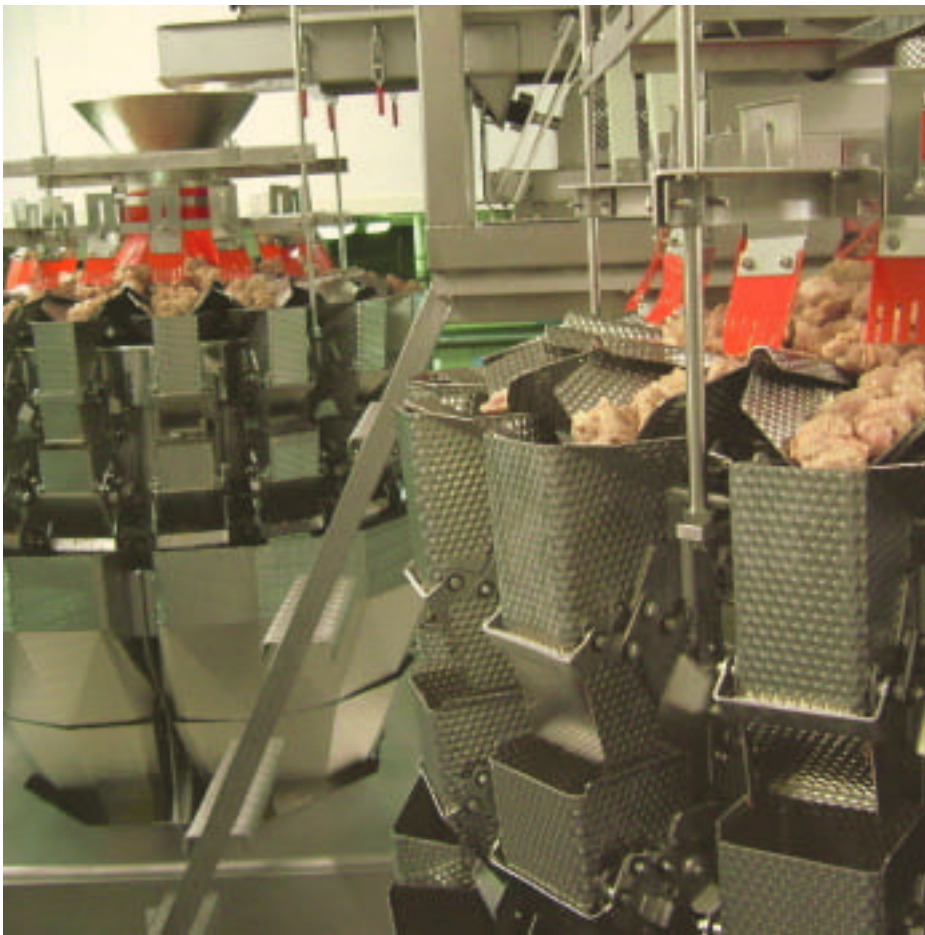
Twin multihead dosing: Ishida system for Saurin, France, provides speeds up to 360 drops a minute
