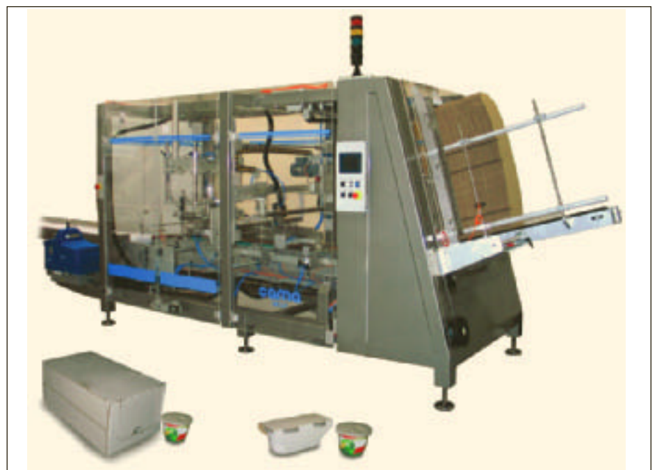
Wraparound case-packing: Cama machine handles multipacked pots at 13-26 cases a minute
