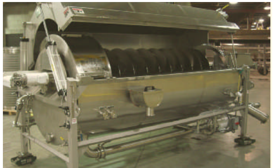
Continuous process: Lyco Clean Flow cook-quench-chill system from BFS Europe uses auger transport
