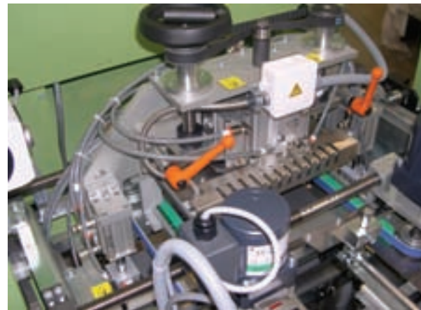
Shrink tightener: Marden Edwards system for end-fold wraps
