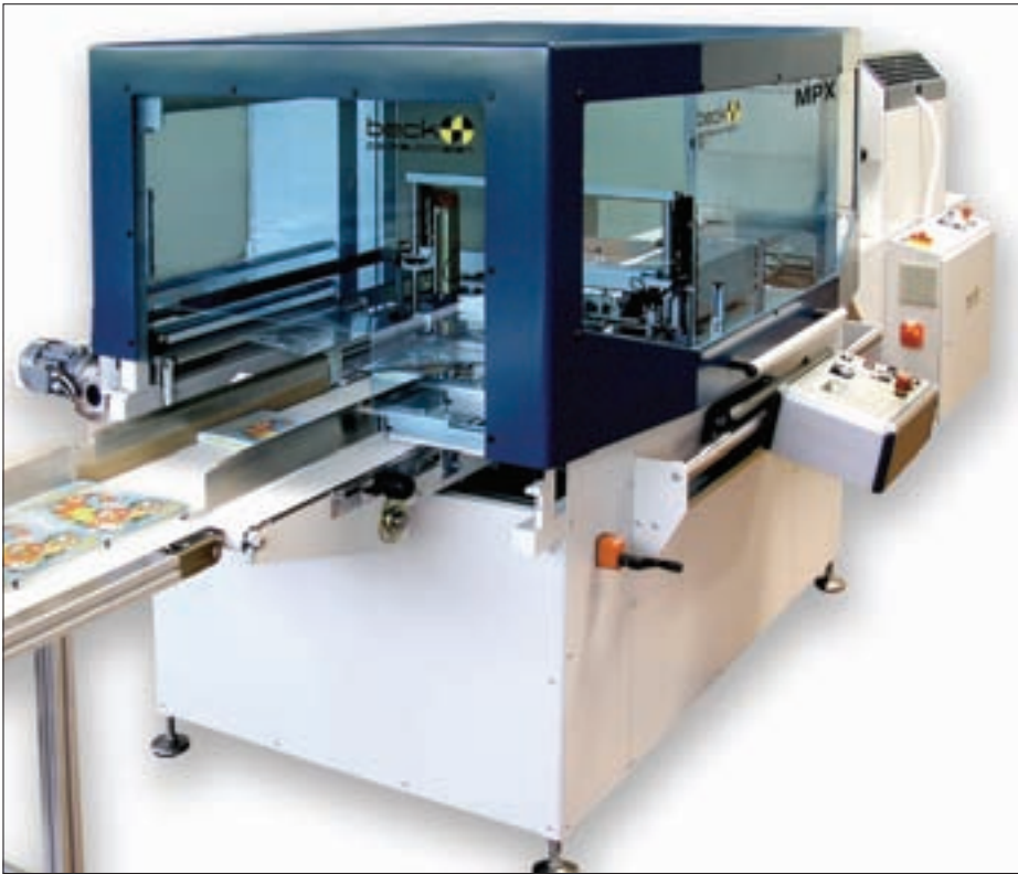
Shrink overwrapper: DVDs and CDs are a principal market for the Beck Multiplex machine
