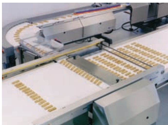
Bradman Lake: The Autowrappers Automatic Distribution System
