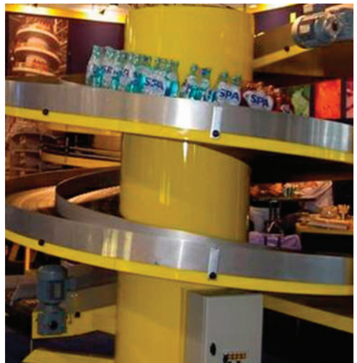
Conveyor Systems: New twin lane Spiralveyor
