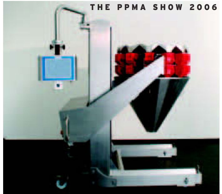
Multipond: Mobile lift weigher can be lowered and cleaned off line
