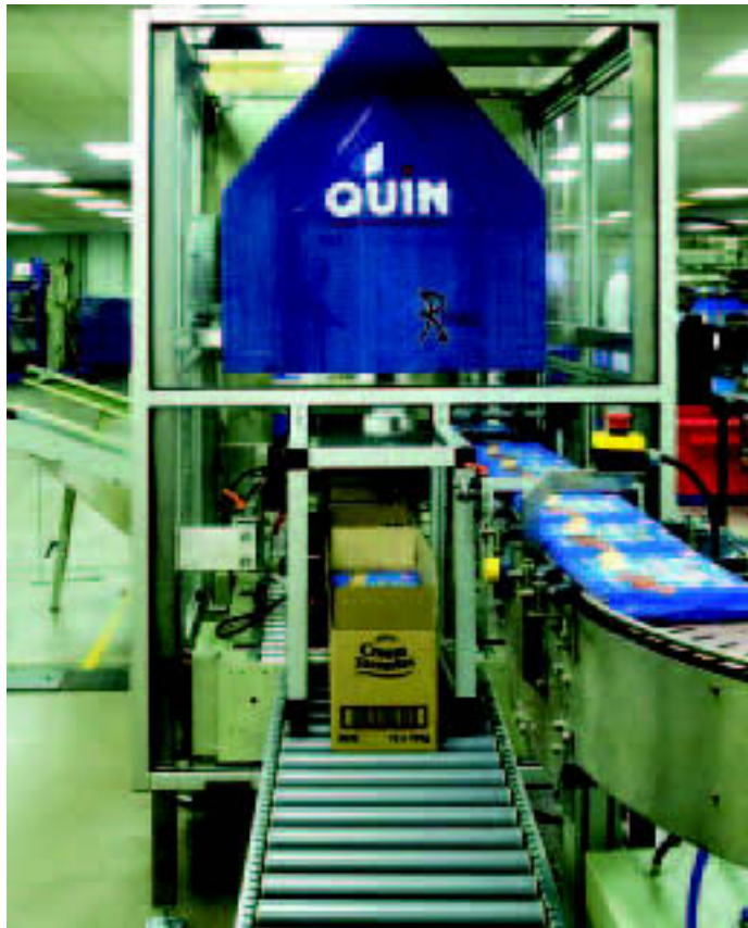
Quin Systems: High speed case packer based on Rtheta product handling
