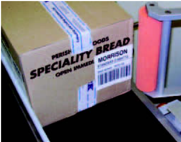
BBK Labelling and Coding: Print-apply for adjacent side case coding
