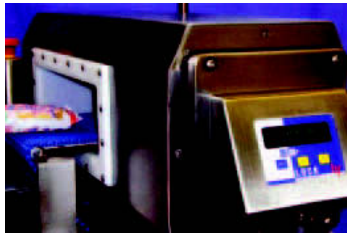
Lock Inspection: Met 30+ metal detector
