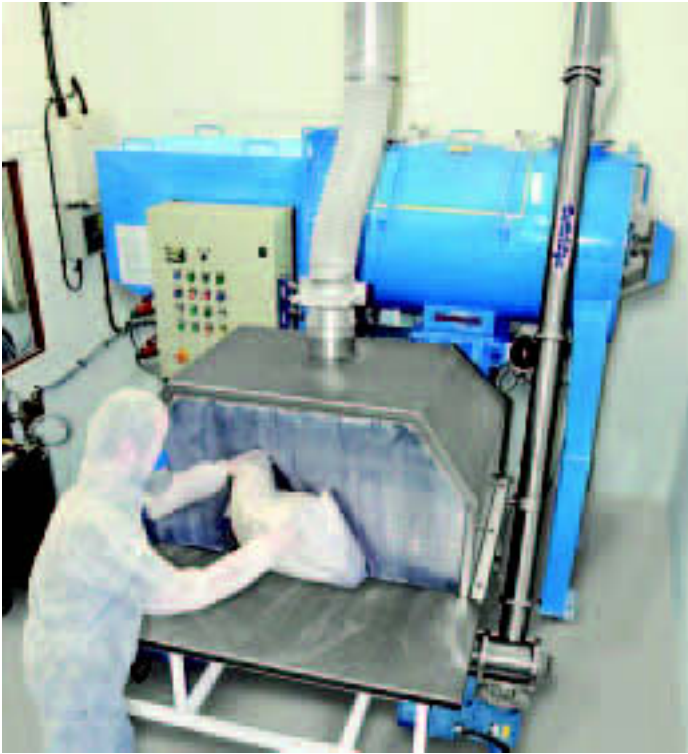
Guttridge Services: Bulkflo loading hopper with extraction to handle garlic
