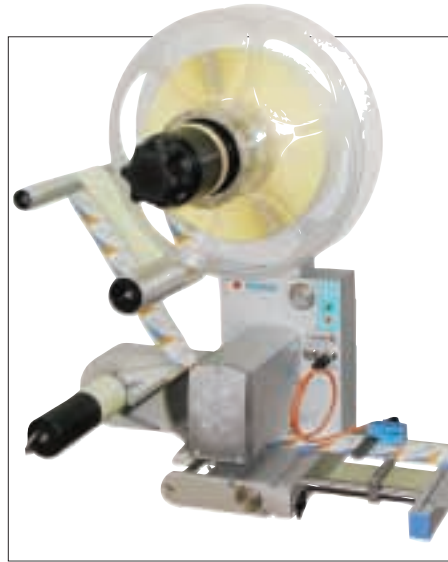
Handling clear labels: Herma 400 Series machines use an inductive label sensor
