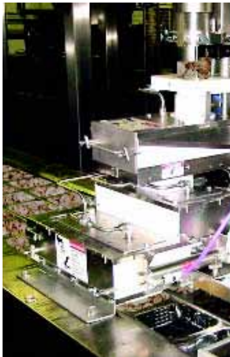
Multi-lane filling: Multi-Fill MPFSC120-01 automatic solids depositor from F Jahn and Co
