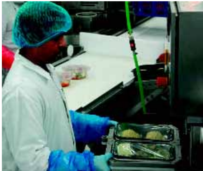
Entry level: Packaging Automation PA182 sealer at Bighams
