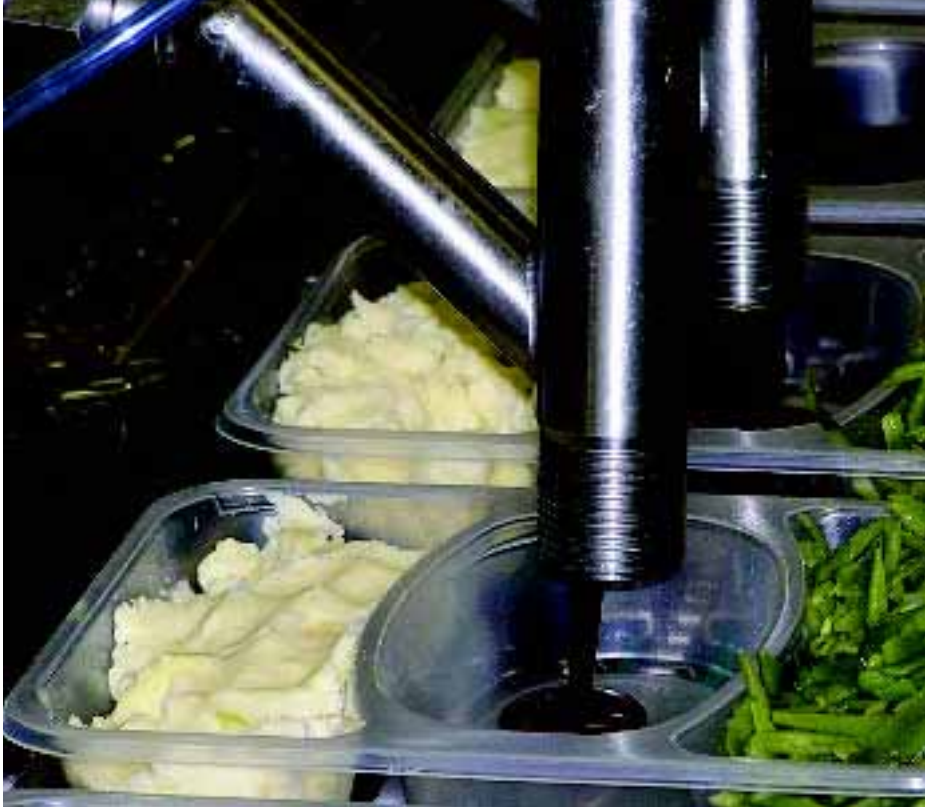
Multi-head filling: Handling sauce with a Turbo Systems depositor
