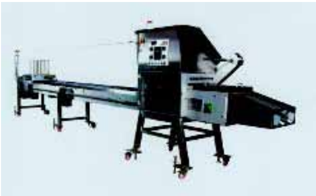
Tray sealing: (top) TS250 machine from AEW Delford for low-to-medium speed production. (Above) High speed twin lane Raque tray sealer. (Left) Proseal AP60 machine will handle up to 160 trays a minute
