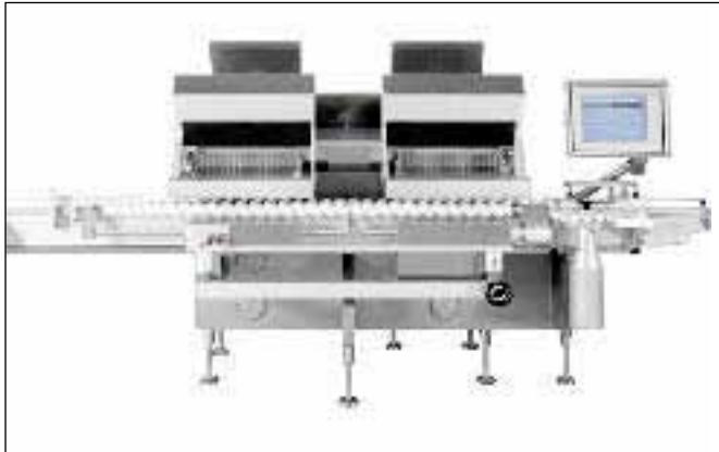
Single tablet rejection: IMA Conta series electronic tablet counter
