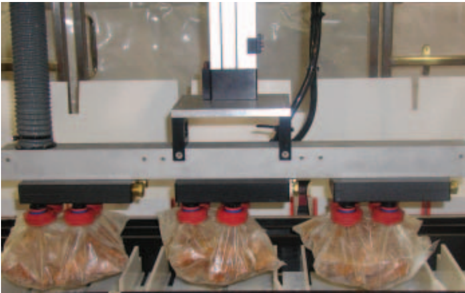
Handling bags of frozen food: Bradman Lake has announced a new robotic top loading machine
