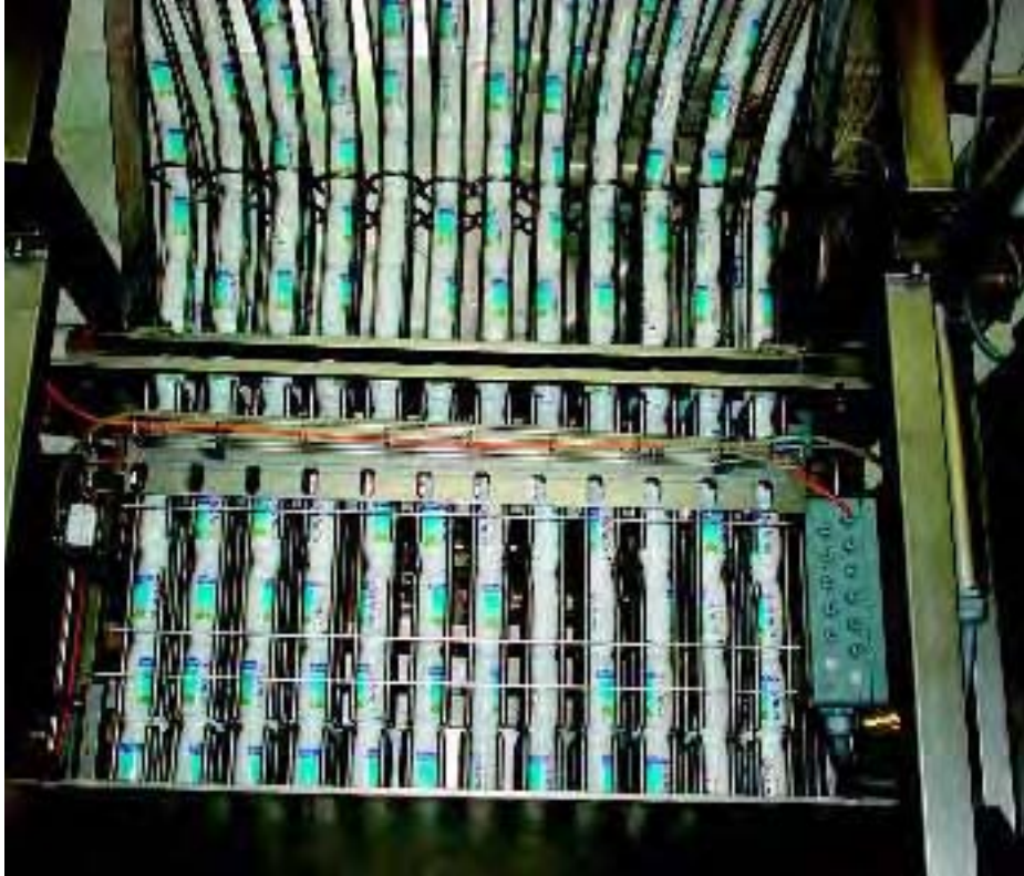
Multi-lane: Hamba Flexline can include up to 14 lanes for speeds up to 50,000bph on 500ml containers
