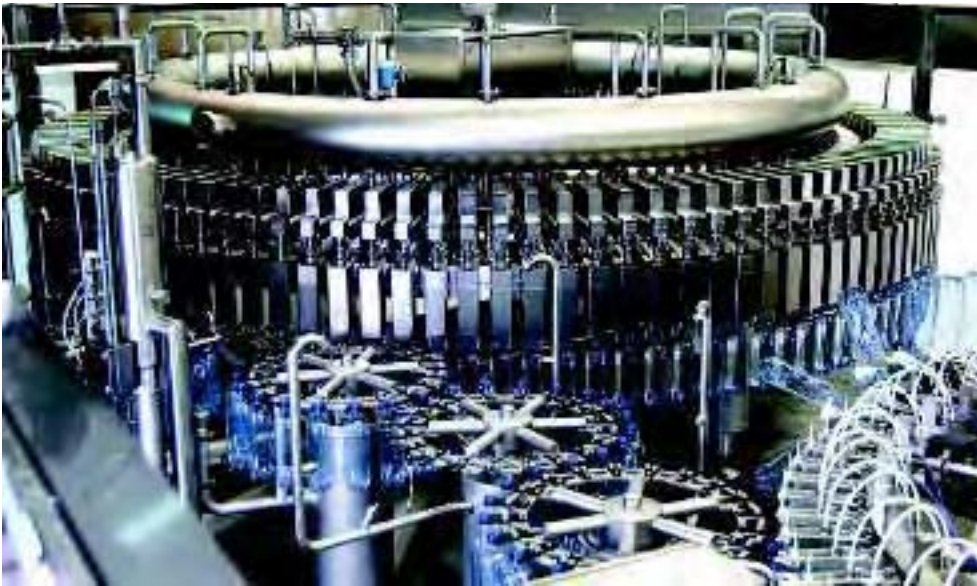
Eliminating the front table: Krones F1 filler breaks new ground in a number of areas
