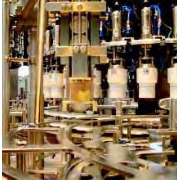
Rotary induction sealing: Fords Packaging and Relco have co-operated to build high-speed rotary induction sealing systems
