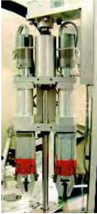
Swing torque head: Cap Coder system gives faster capping
