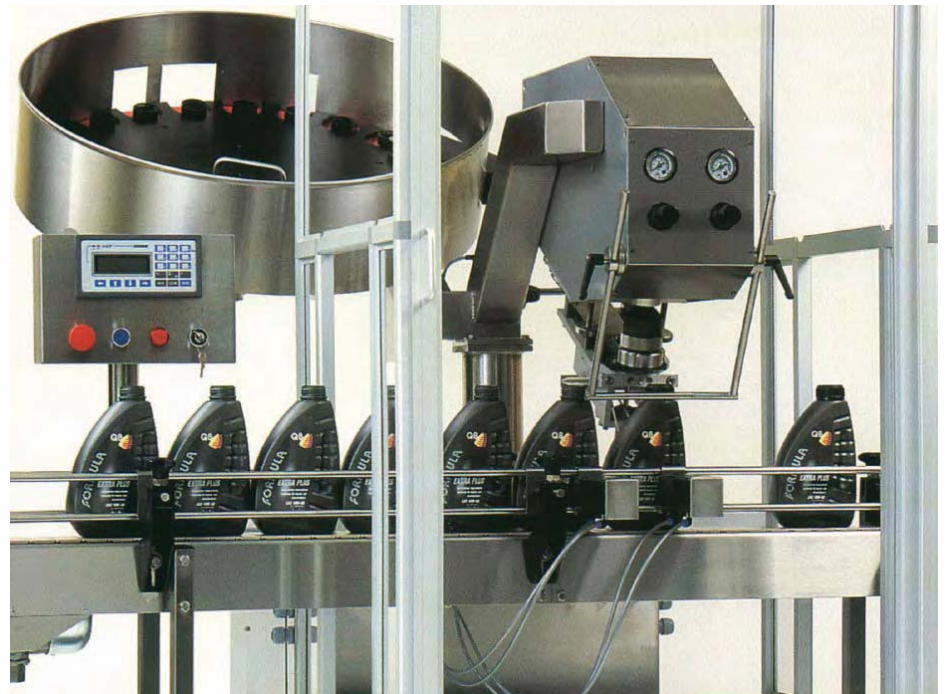
Swedish capper: The EC40 is among Fillpak cappers now available in the UK from SP Filling Systems
