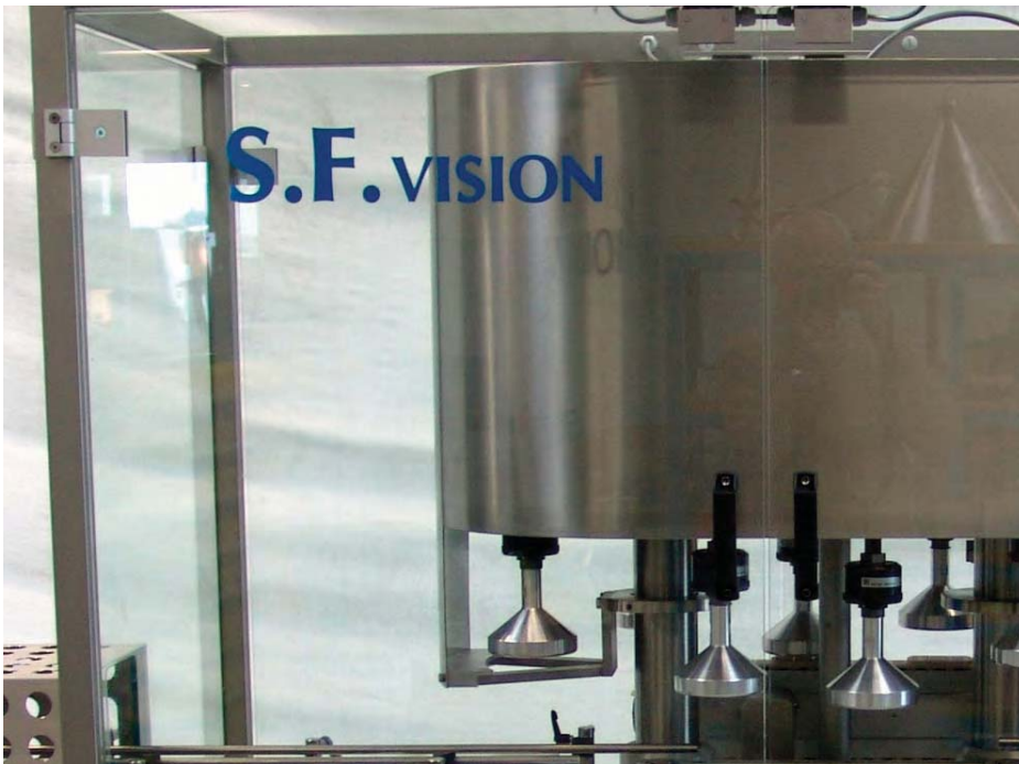
Saving space: Containers and capping heads follow an oval path on the SF Vision machine
