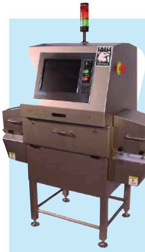
Combination X-ray machine: Eagle Combo from Smiths Detection incorporates a checkweigher
