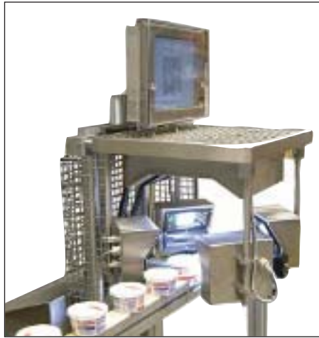
Checking lid against container: Dimaco Veri-ID vision system establishes the identity of both
