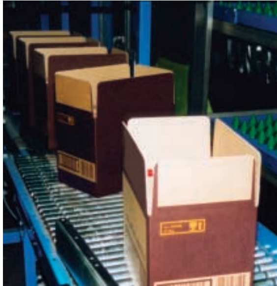
Turning cases: CSL system feeds case-packers at distillery
