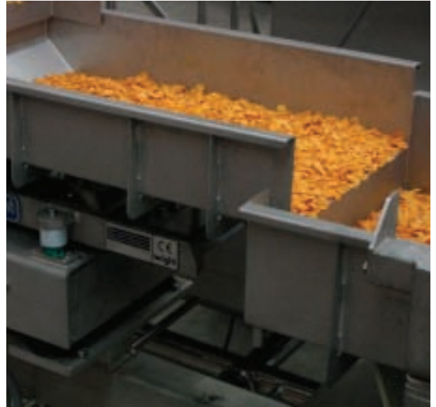
Easy to clean: Weighwright vibratory weighing conveyor
