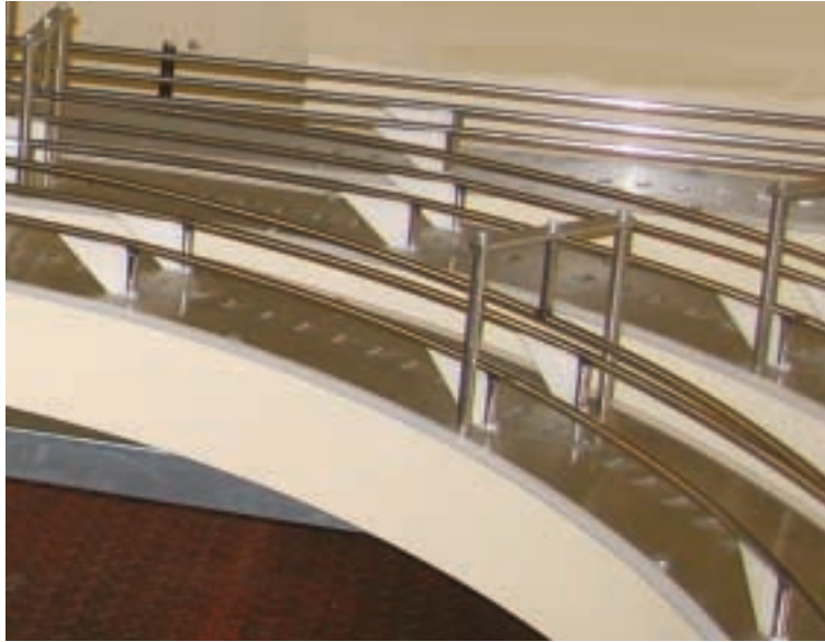
Air conveyor: Sewtec's new system handles cartons at high speed
