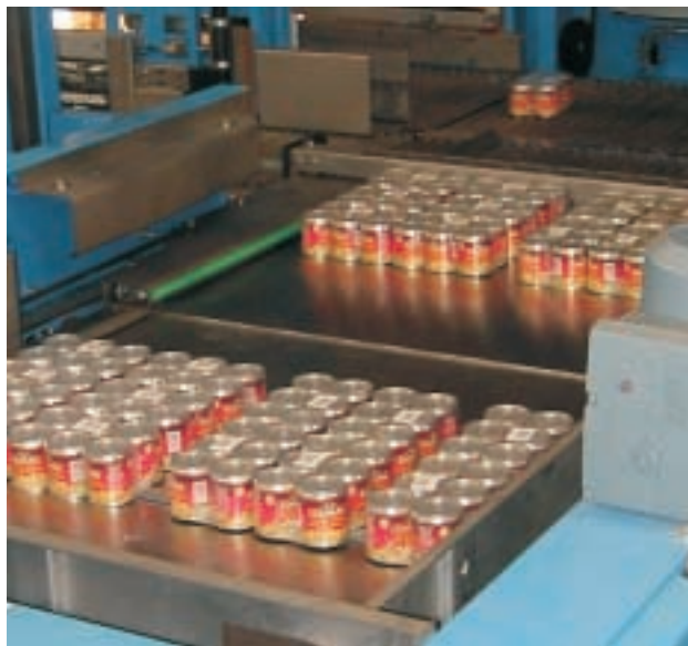
Cans without trays: C-5000 palletiser from CSi handles vulnerable packs
