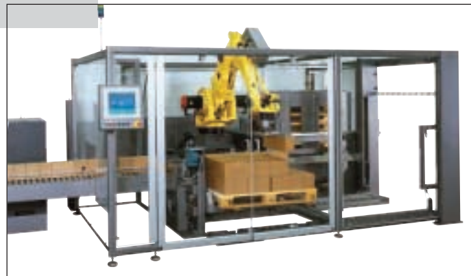
Robot palletisers: Top: Ivanhoe I-Pal is delivered in a container and can be quickly installed. Above: IMA Flexpalletiser operates at 15 cycles a minute
