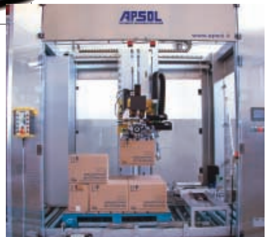
Pick and place palletisers: Top: Euroimpianti Skilled 101 operates in 9sq metres. Above: Apsol CP-G can handle a 40kg payload
