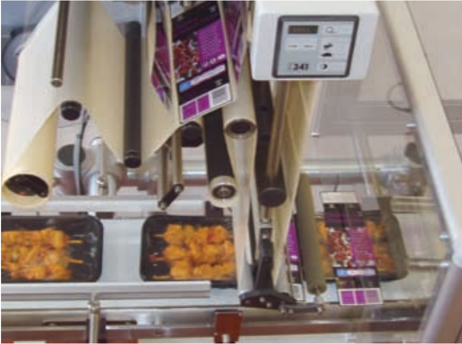
Labels in place of sleeves: Tray-fix applicator developed by Advanced Labelling Systems
