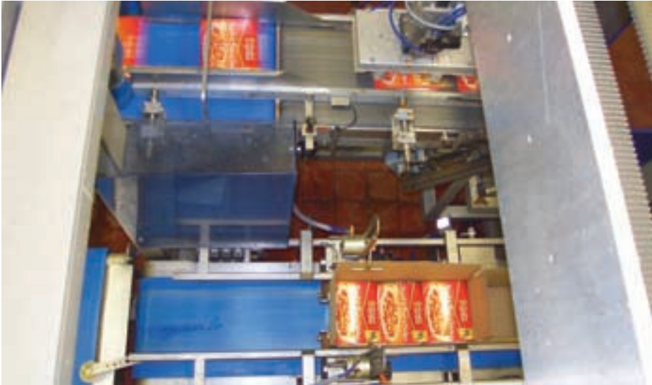
Pick-and-place: BluePrint HOP case-packer at Oriental foods handles 70 trays a minute
