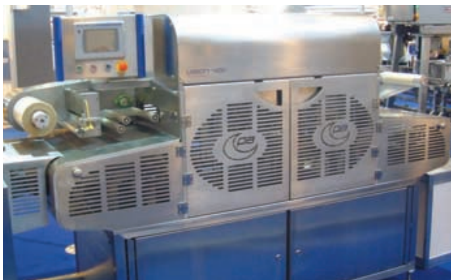
Quick changeover: Vision 400 tray sealer from Packaging Automation
