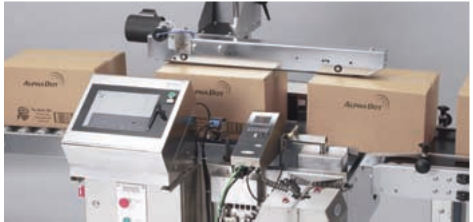
Multiple coding: Alpha Dot's Multi system can print on both sides of the case
