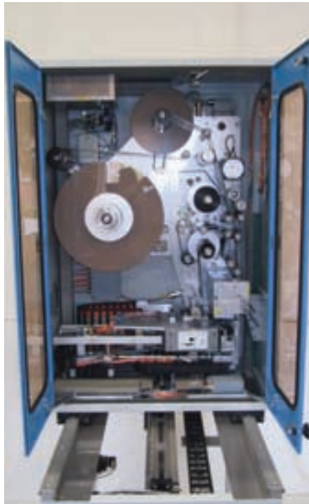
Pallet labelling: New Logopak 920PFM machine can handle 150 pallets an hour
