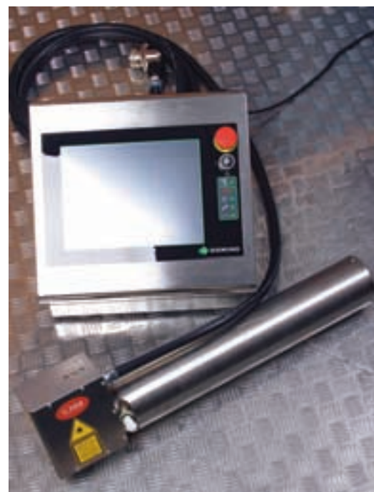
Scribing laser: Compact Domino S300 is able to code 1000 PET bottles a minute
