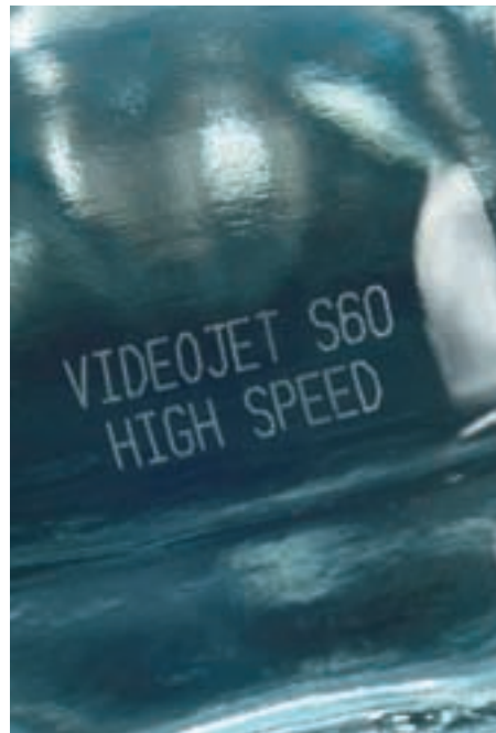
Steered beam: Print from the Viodeojet S60 laser coder can be read by vision systems
