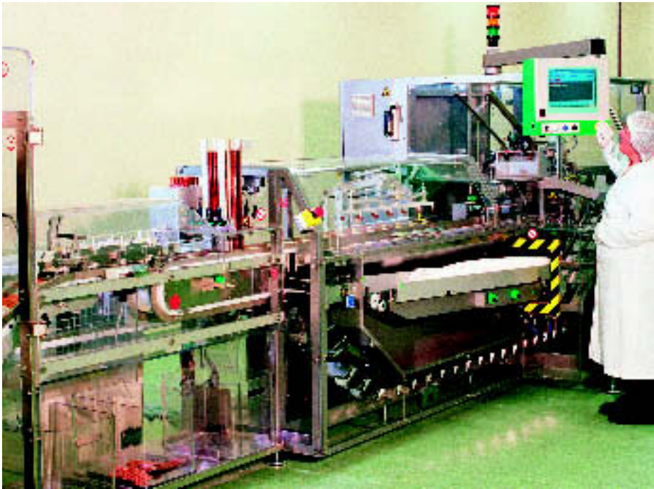
Expanding production: Surepharm has installed a Marchesini MB430 blister packing line
