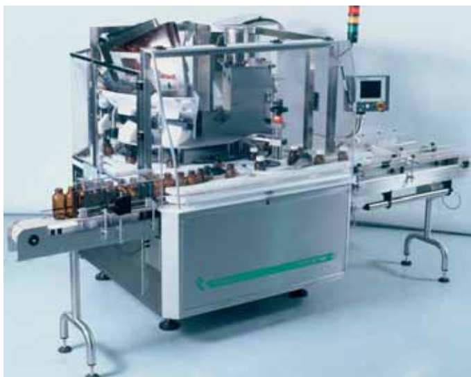
Positive separation: Bosspak machines use rotary sorting disks to separate tablets and capsules. Below: The new Bosspak RTC 80 MB machine for medium speed duties
