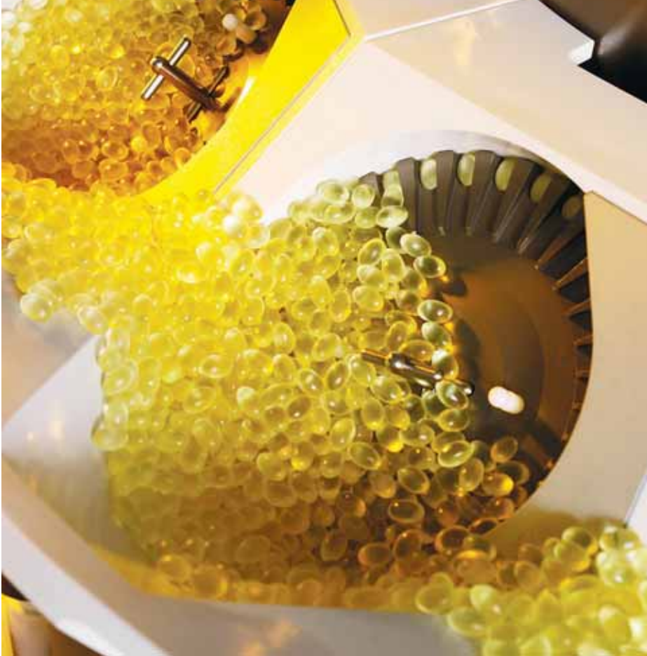
Positive separation: Bosspak machines use rotary sorting disks to separate tablets and capsules. Below: The new Bosspak RTC 80 MB machine for medium speed duties
