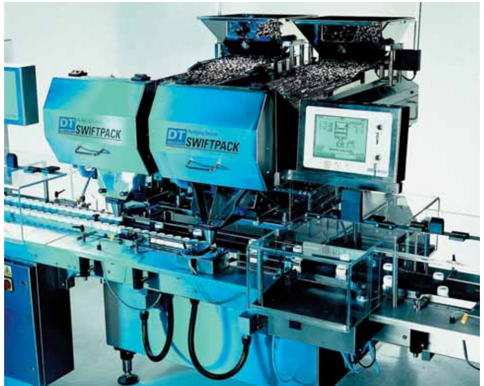
Extra inspection: Swiftpack SV2 uses an electrostatic field to check tablet and capsule quality
