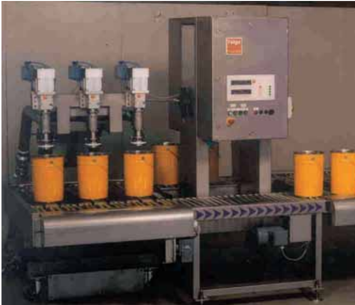
In-line step-across: Feige Rapid Filler can have up to six filling valves
