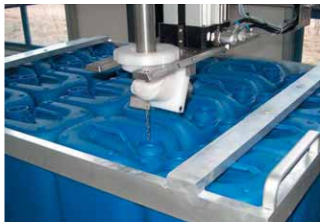
On-pallet drum filling: Top: Systems from Permex are able to fill multiple layers of containers. Left: Automatic system from Feige uses a camera to locate the bung holes. Above: The Logdos Teach-In system can be used with a template so that only one or two sets of co-ordinates need be given
