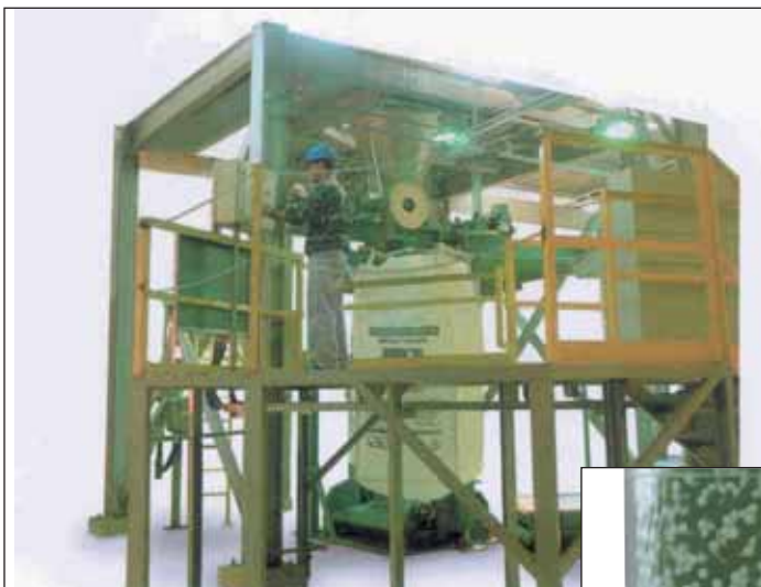
Above: Latest version of the Flowmat Carousel bag filler has automatic final weight adjustment.
