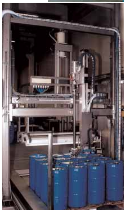
On-pallet drum filling: Top: Systems from Permex are able to fill multiple layers of containers. Left: Automatic system from Feige uses a camera to locate the bung holes. Above: The Logdos Teach-In system can be used with a template so that only one or two sets of co-ordinates need be given
