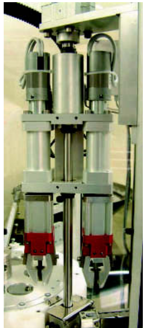
Swing torque head: Cap Coder system gives faster capping for bigger bottles
