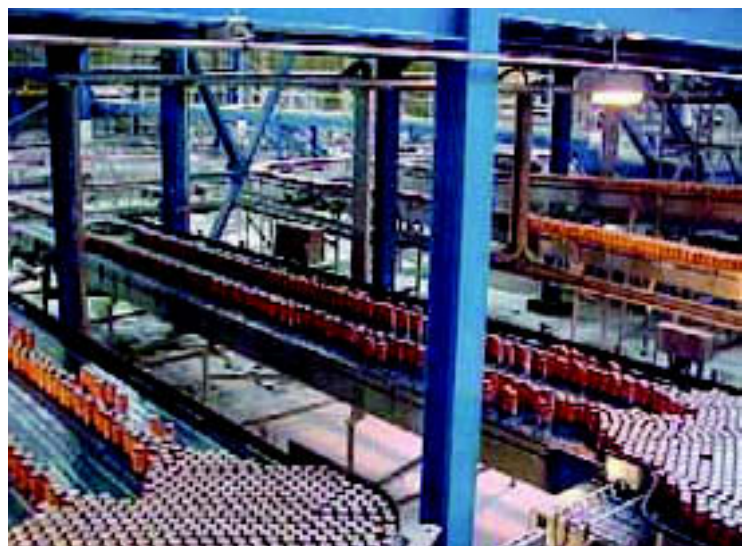
Handling full cans: Filled cans are taken to a new two deck pasteuriser
