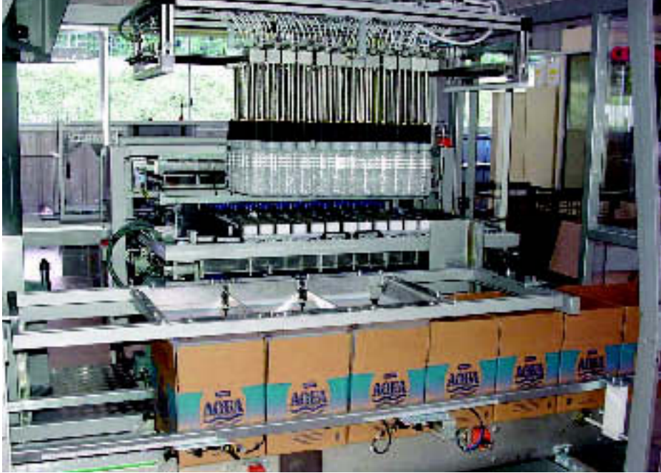
Pick and place: High output top load case packer from Cermex
