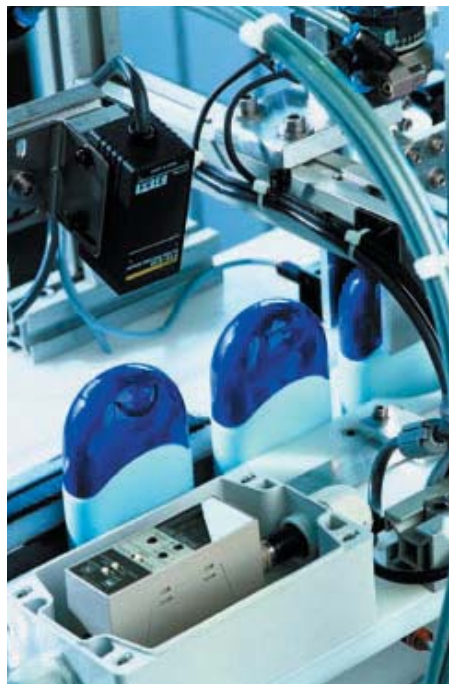
Typical inspection point: An application for Omron's F10 pattern matching sensor
