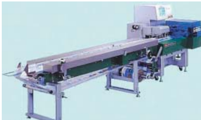
Handling sticky products: Omori bottom-reel machine from Selo-Bollans
