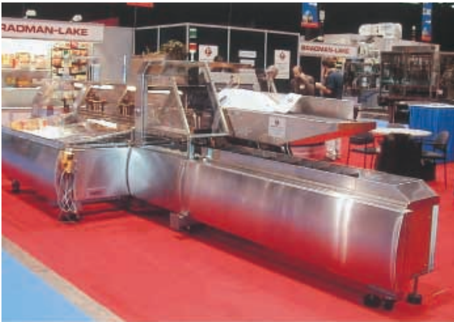
Nine servo drives: Bradman-Lake's first 100 per cent servo driven end-load machine, the SL9000
