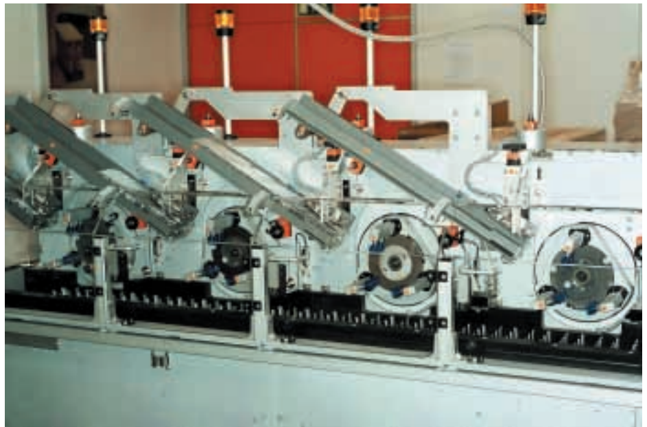
Blister feeding: Four station blister feeder designed by IWKA for the Cartopac SC4 machine
