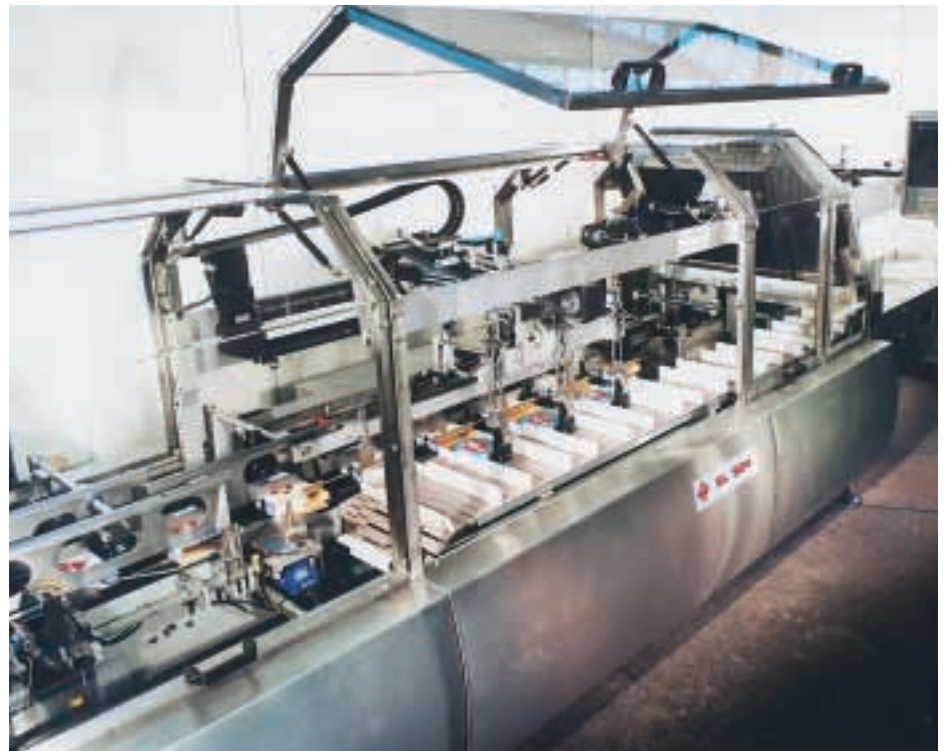
Robot loader: Bradman-Lake SL904 with overhead robot inserter. A smaller footprint is one advantage
