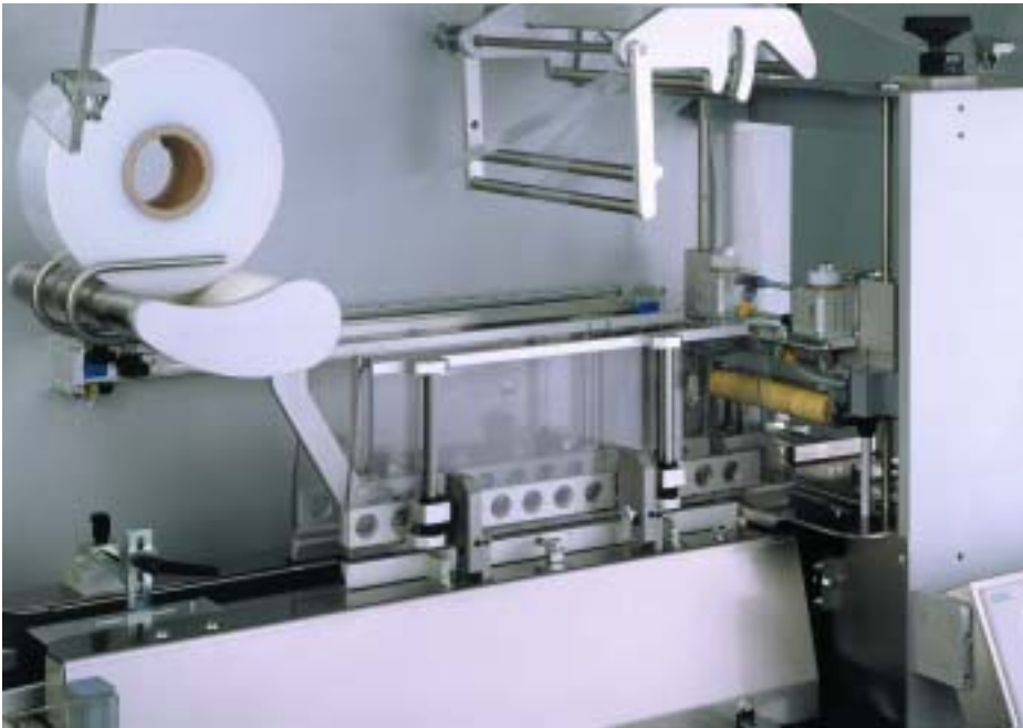
Stretchbanding for bundles: Auto Skinnetta machine from Propack Automation
