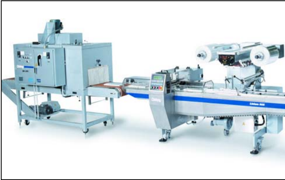
Shrink film flow-wrapping: The new Linium 305 machine from SIG Doboy
