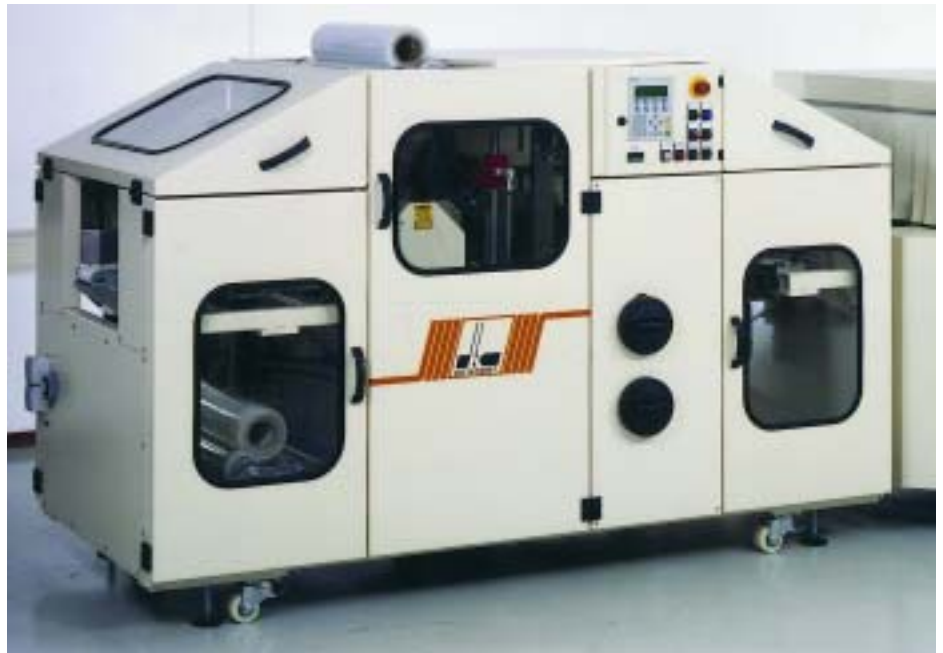
Four-side seal: Europack EPS4 offers flexibility to handle a variety of products
