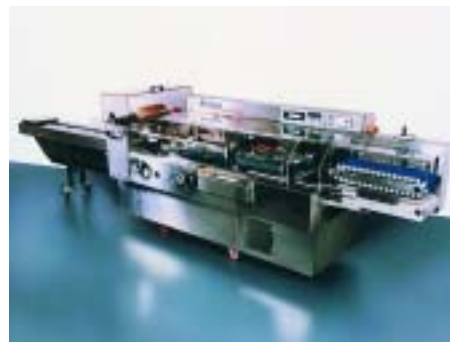
Tray overwrapper: Delford SP6000 can handle up to 90 trays a minute
