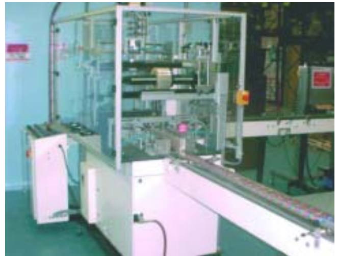
Condom carton wrapping: Paladone Products, Shoreham-by-Sea, has installed this Sollas 20 end-fold overwrapper
