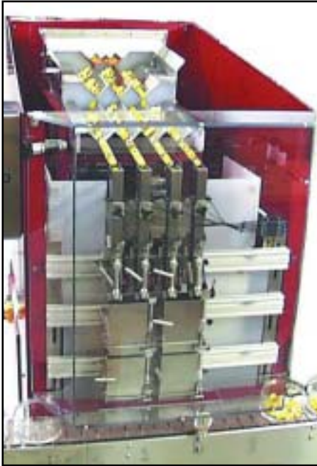
Handling small items: Palace vibratory oscillating tray counter from Burge Equipment
