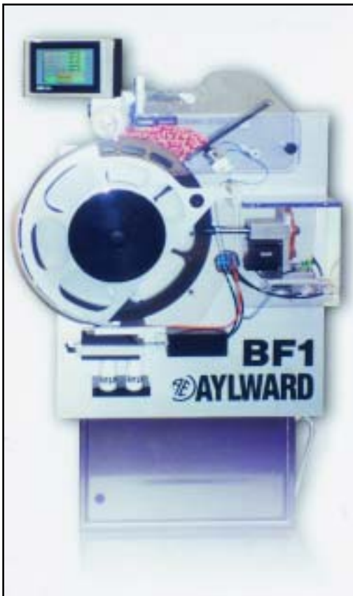
Rotary feeding: Aylward counters can be built with up to 30 wheels, each giving 1000 a minute
