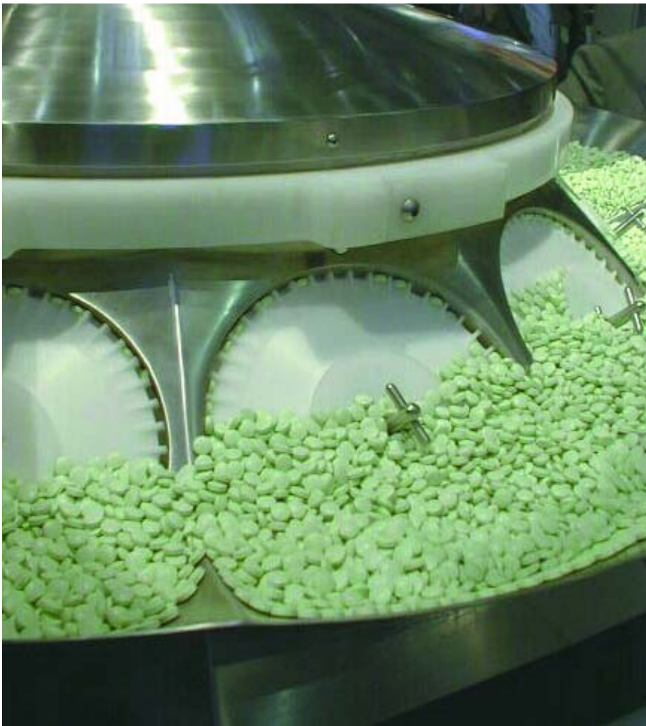
Separation by disks: Bosspak RTC 200 provides speeds up to 200 x 100-count containers a minute
