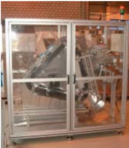
Compressing bags: NCP 220-400 case packer from Nor-Reg handles 35 cases a minute
