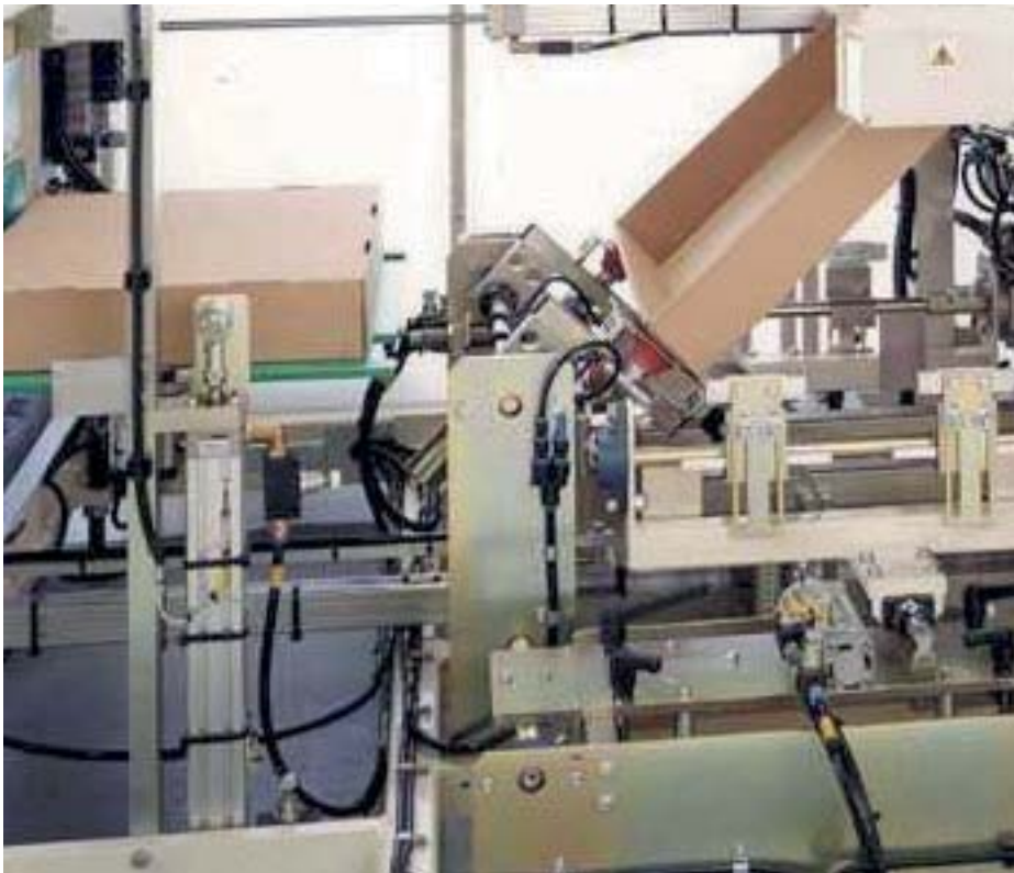
Tray and lid erector: Europack machine built with vibrating table for M & H Plastics
