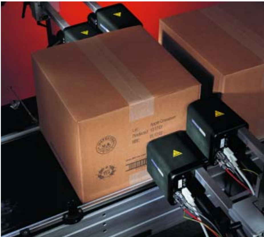
Touch dry: Markem's new 5400 ink jet uses touch dry hot melt inks. Up to four beads can be controlled
