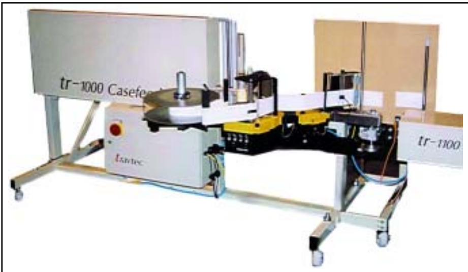
Labelling case blanks: Travtec TR-1000 case feeder can be equipped with a labeller and bar code scanner
