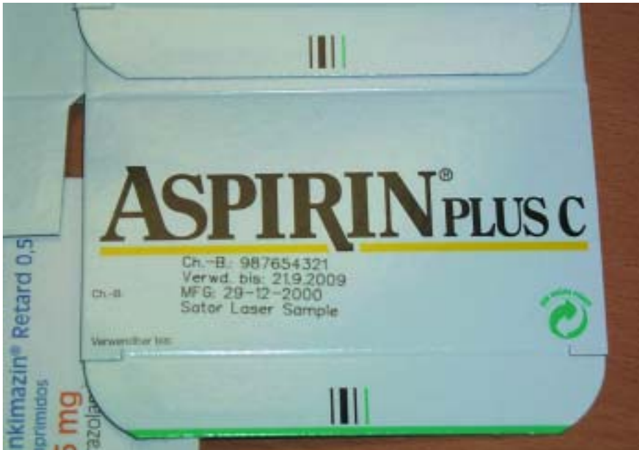
Vector laser: Code on white pharmaceutical carton produced by the VisioMark system
