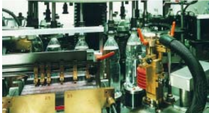
Paper or plastic: Innoket Roland can handle both labelling media
