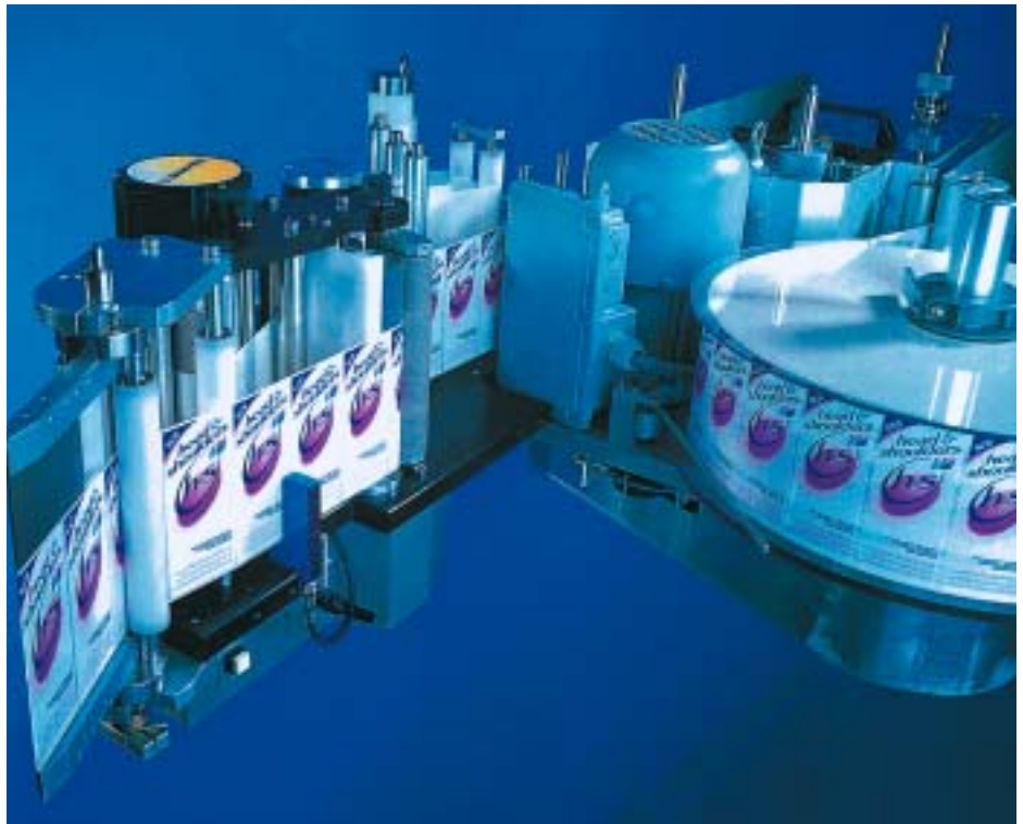
High performance: Pagomat 6HL operates at speeds in excess of 1000 labels a minute
