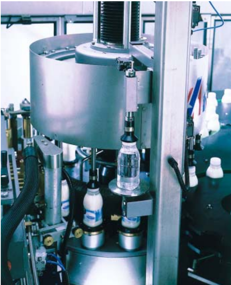
Changing bottle height: KHS Anker system uses a sample reference bottle on the external platform
