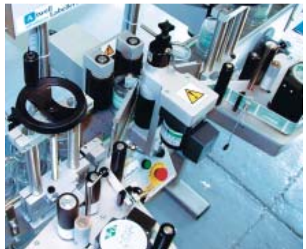
Front and back: Tri-Roller from Atwell reverses direction to apply the back label, avoiding the need for registration marks
