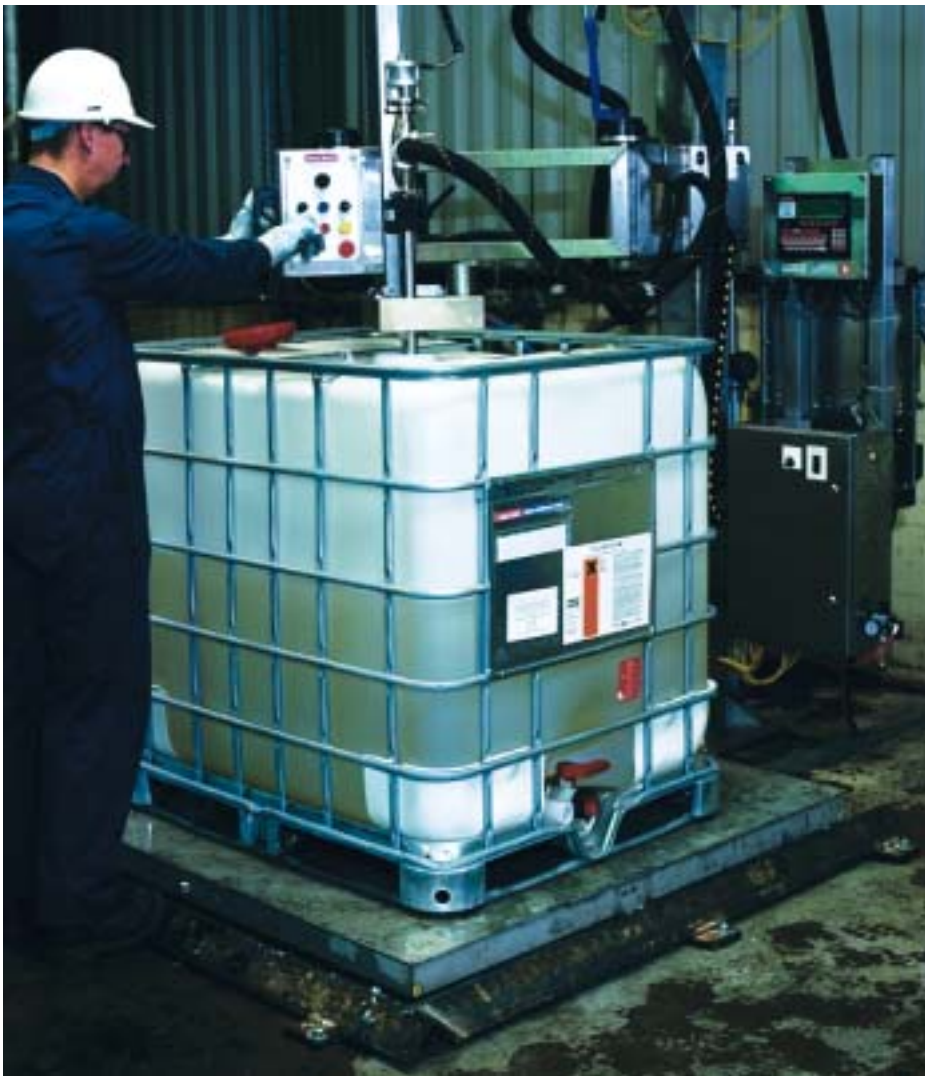
Gravimetric range: Avery Berkel supplies systems for single or multi on-pallet containers up to IBCs
