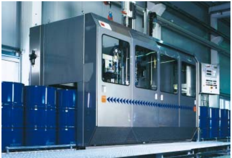
Filling hazardous chemicals: A Feige Type 84 in-line drum filler is being used by Atofina UK
