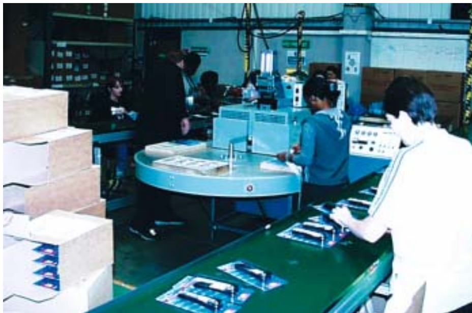
Output doubled: Rotary blister sealer from Relco at Apex Retail Distribution
