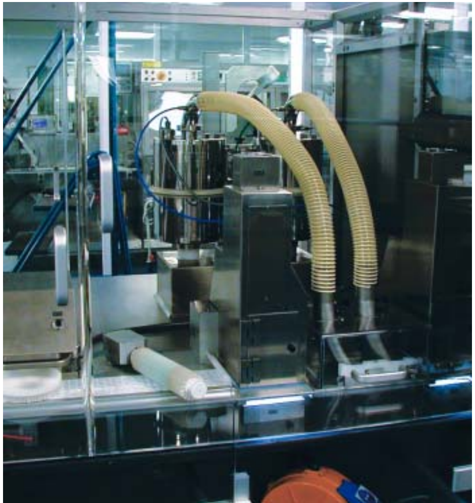
On-machine tablet recovery: IMA C90 at Alpharma empties incomplete blisters for tablets to be re-used
