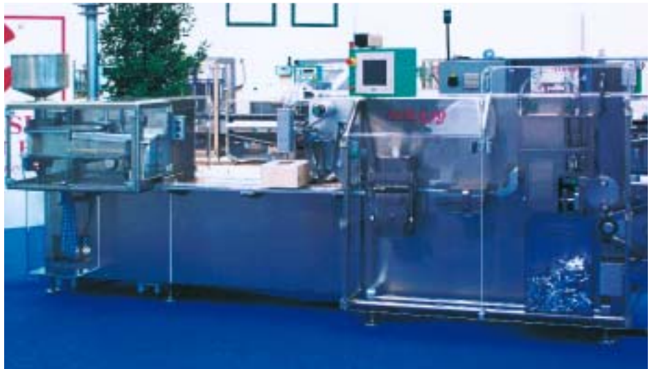
Integrated line: Blister packing section of the Marchesini MB430 blister packing/cartoning line
