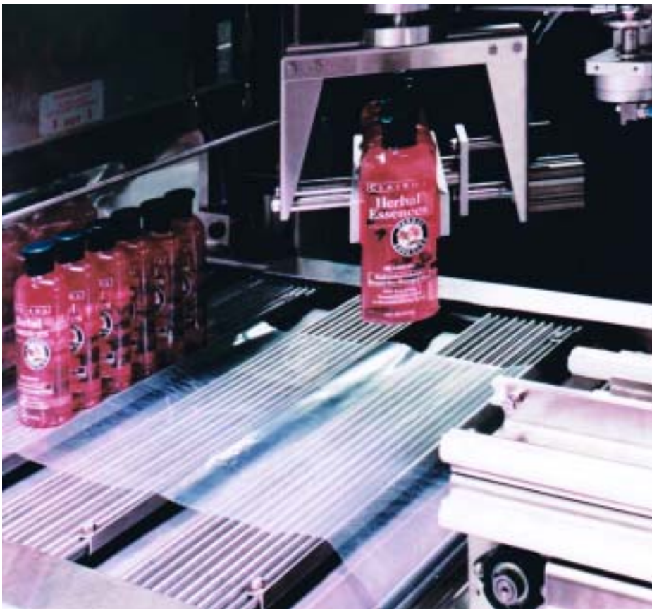
Pick-and-place: Polypack Rokb system places unstable product directly on to the film
