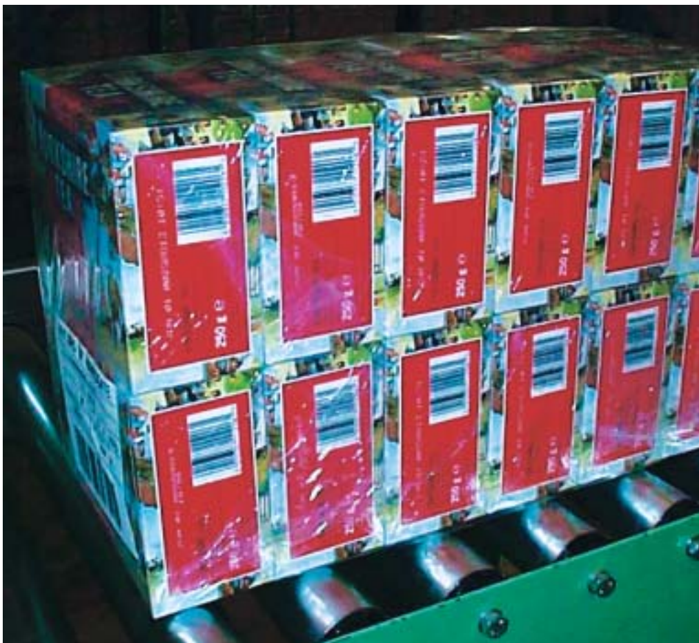
Folded at the side: The Meurer approach to creating completely enclosed packs
