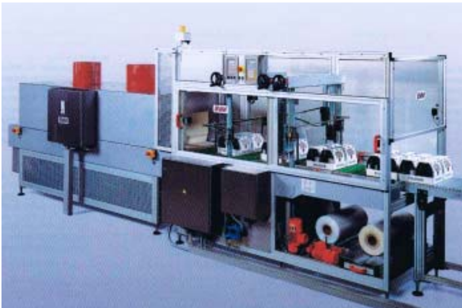
High speed: BVM Speedmaster machines from Wrapid Packaging can reach 100 trays a minute
