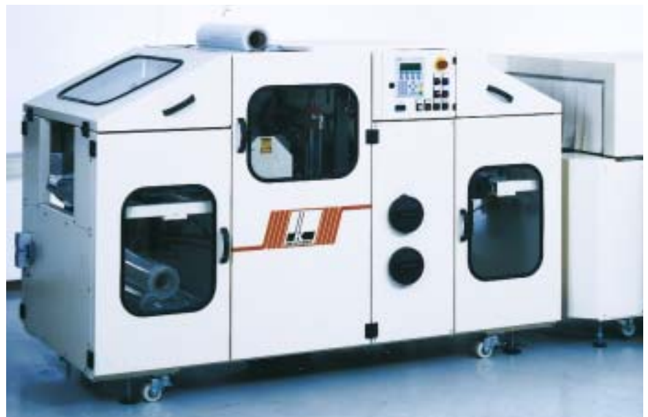
Enclosed packs: Europack's new EPS4 twin reel machine also seals the film at the pack sides
