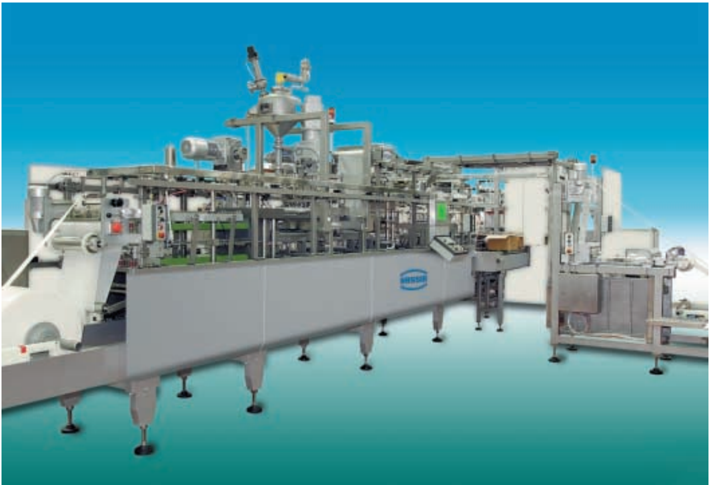
Producing and filling dual cavity pots: A Hassia THM 1842 line is being installed for a UK customer by agent Engelmann & Buckbam Machinery
