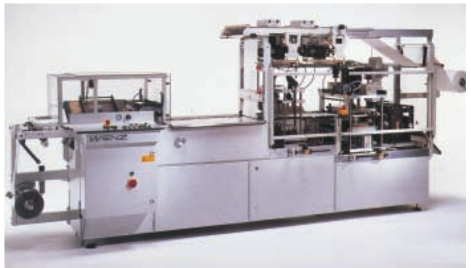
Medical products: Wenz WM230 thermoform-fill-seal blister machine from Soudal
