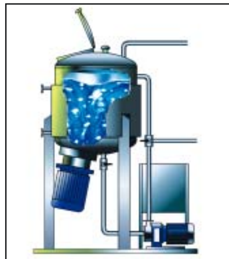
Silverson reclamation system: stage 1: Materials are circulated through the bottom entry mixer until they are reduced to granular size
