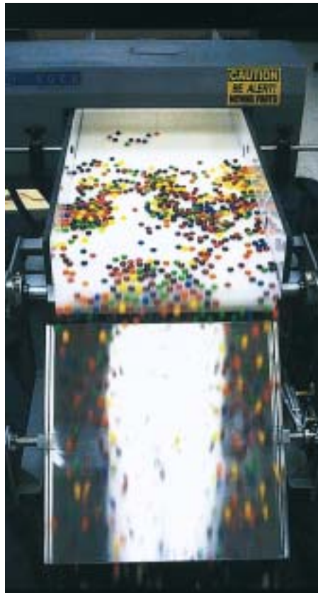
Pre-packing inspection: The Lock Met 30+ conveyor based metal detector
