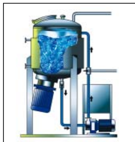
Stage 2: The in-line mixer is brought into action subjecting the material to intense high shear
