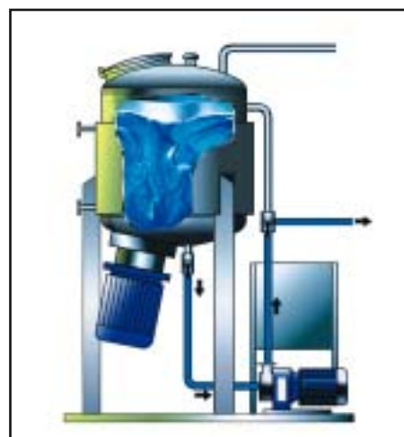
Stage 3: The in-line mixer is used to pump the processed rework back to the production line
