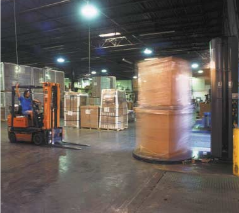
Pull for service: Lanyard switch allows fork truck driver to start the Lantech Q300XT from his seat
