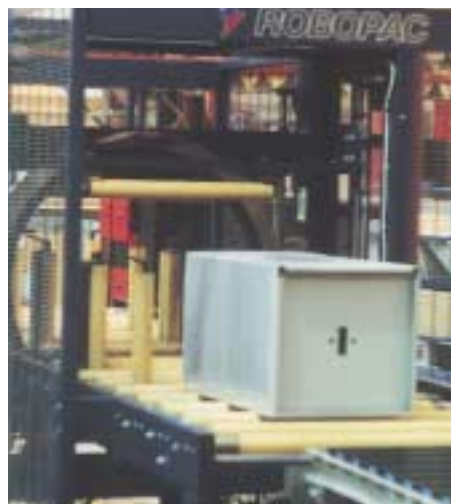
Horizontal wrap: Small filing cabinets are handled on a Robopac Spiror machine
