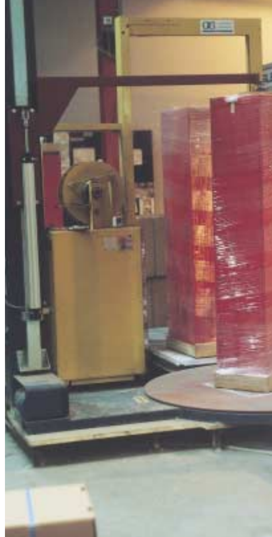
Single wrap for lockers: Rotoplat 505 semi-automatic wrapper can handle 30 a minute
