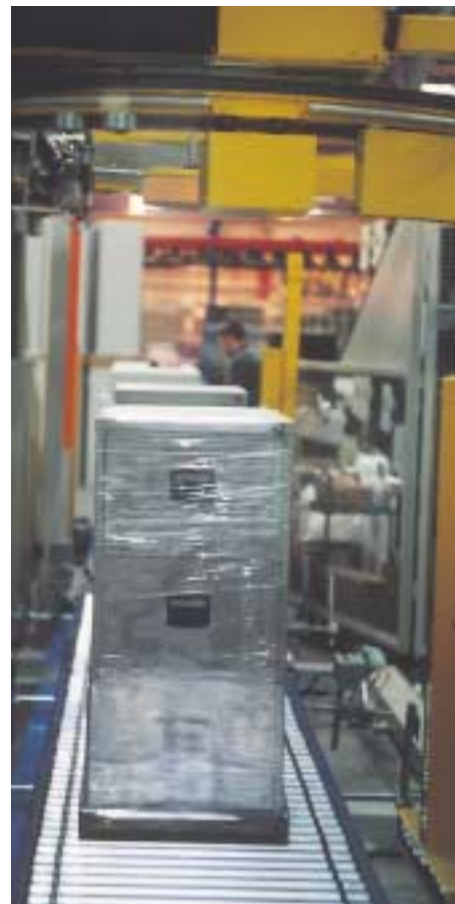
Higher speed: Robopac Genesis ring wrapper handles a filing cabinet in less than 40 seconds
