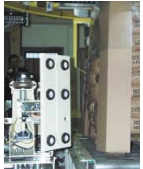
Extra corner strength: Automatic corner post applicator on the Mancon 2200 ring wrapper
