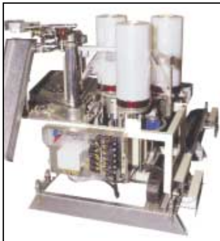
Auto reel change: The Genesis ring wrapper can be equipped with an automatic film reel magazine
