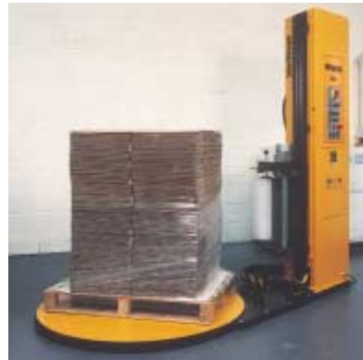
Photocell height sensing: Upgraded Strapex Delta has additional features as standard
