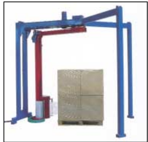
Wrapping at floor level: The Mimi 041 semi-automatic rotary arm machine from S&B
