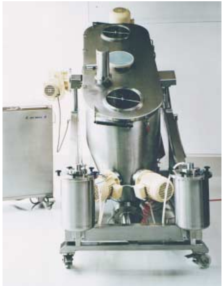
Inclined for productivity: Prodim mixer for powders
